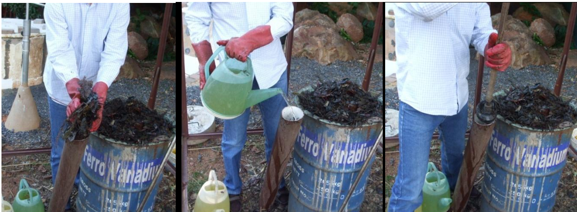
Figure 3 – Loading biomass into the inlet pipe. The procedure is to push few handfuls of biomass into the pipe, followed by water, followed by using the plunger to push the load own into the dome chamber.
