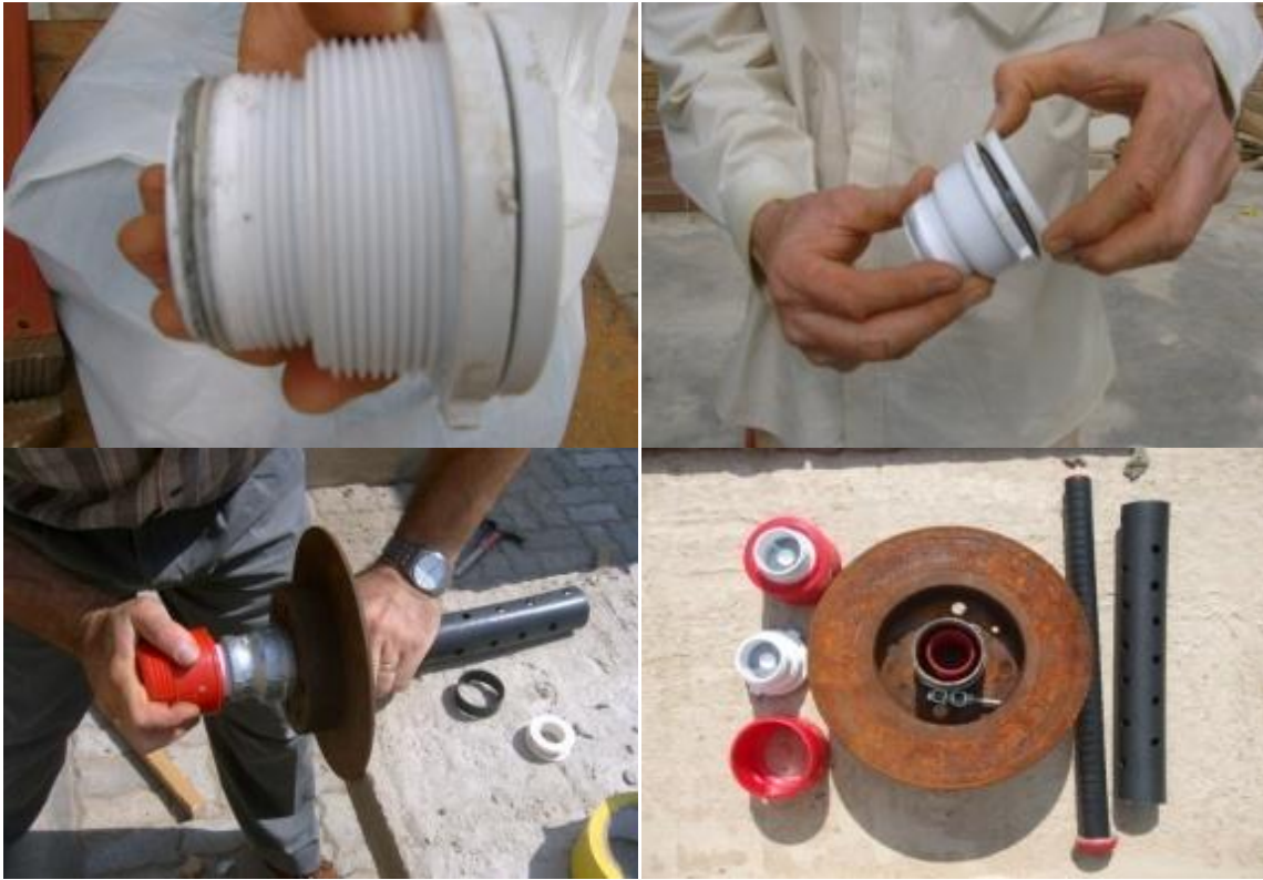
Figure 3 – Moving clockwise: In (a) the valve is shown in its closed configuration, in (b) it is shown open, in (c) the various components of the valve may be seen, while (d) shows the components in their assembled configuration.
