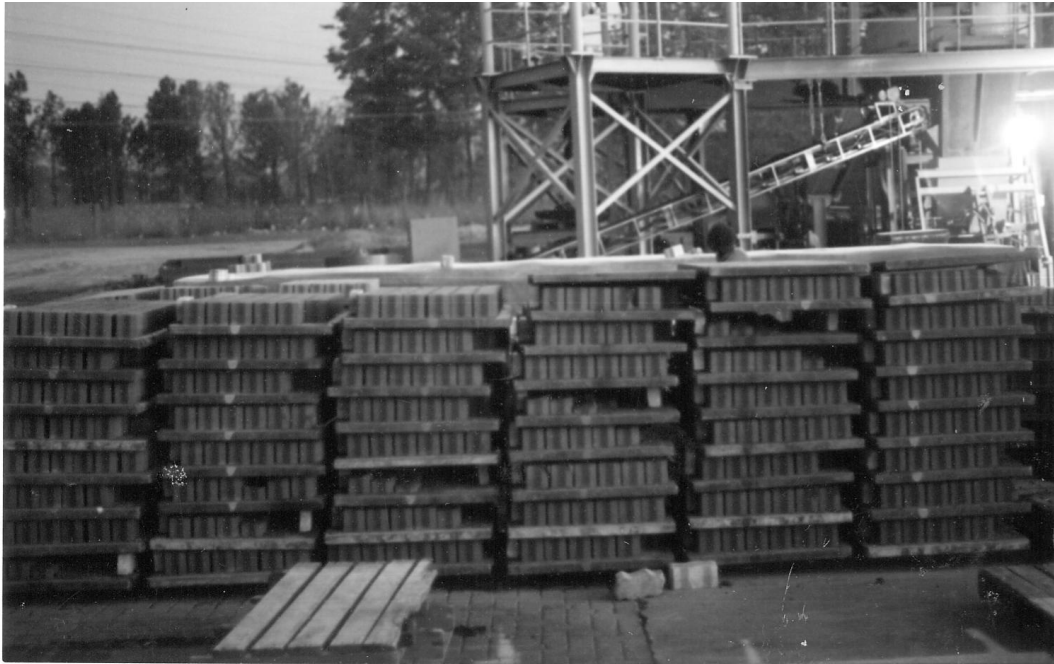
Figure 3.9 The pallets were marked with different paint colours to identify the various mix designs (the blocks could not be marked at this stage since they were still wet)
