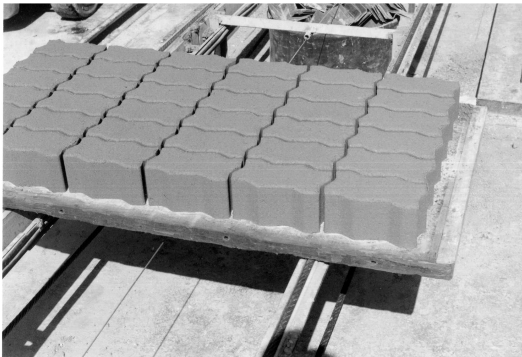
Figure 3.7 After moulding, the blocks are ejected from the block machine onto a rope conveyor
