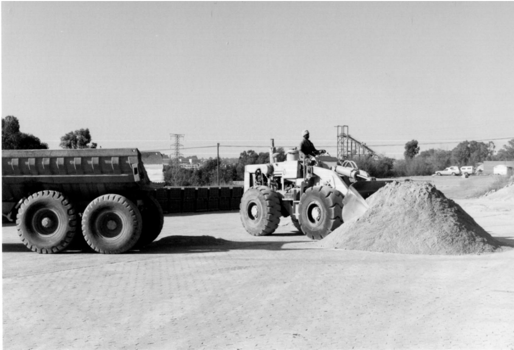
Figure 3.2 Blending of the sand to ensure uniformity
