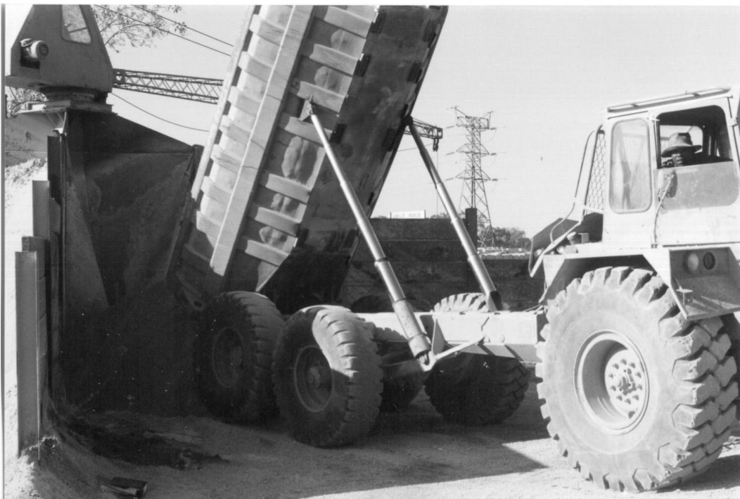
Figure 3.3 Sand being loaded into aggregate bin No. 2
