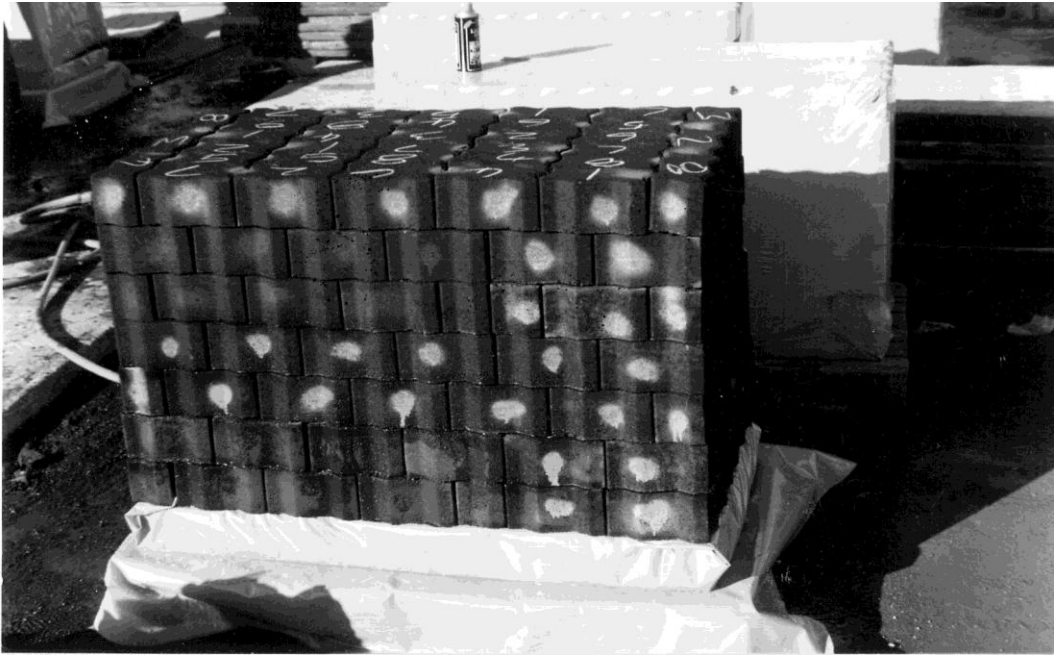
Figure 3.12 Blocks destined for the laboratory are numbered on their upper faces from one to eight
