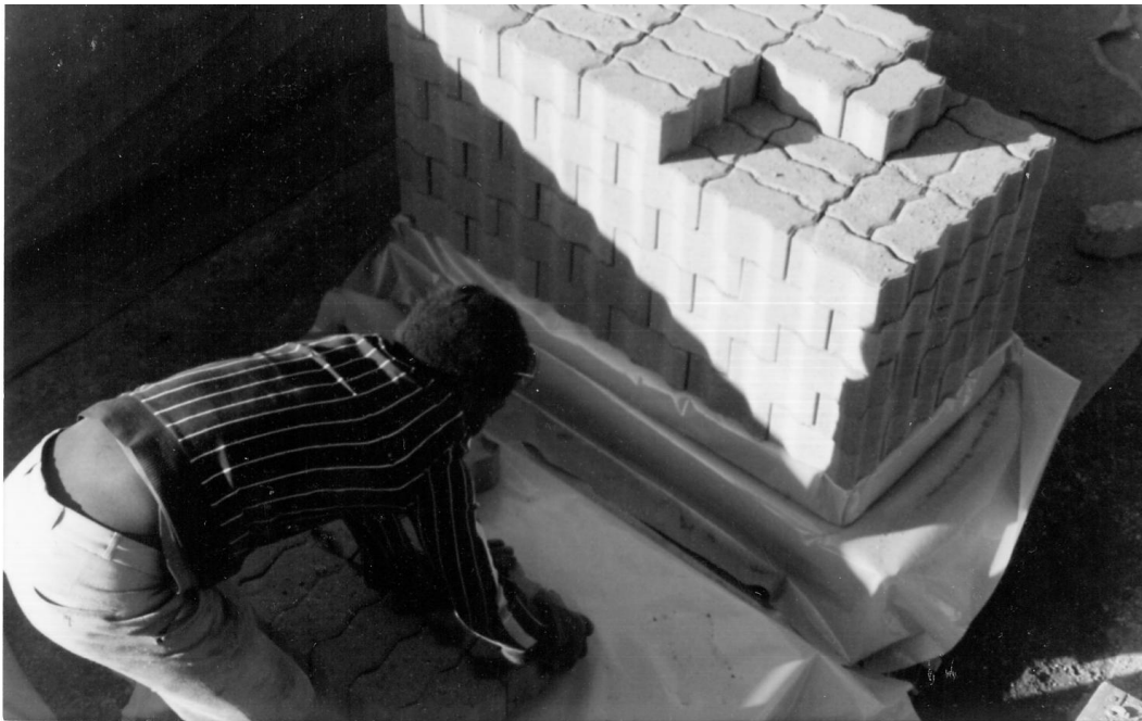
Figure 3.11 The blocks were hand packed and sealed in a double layer of shrink-wrap plastic
