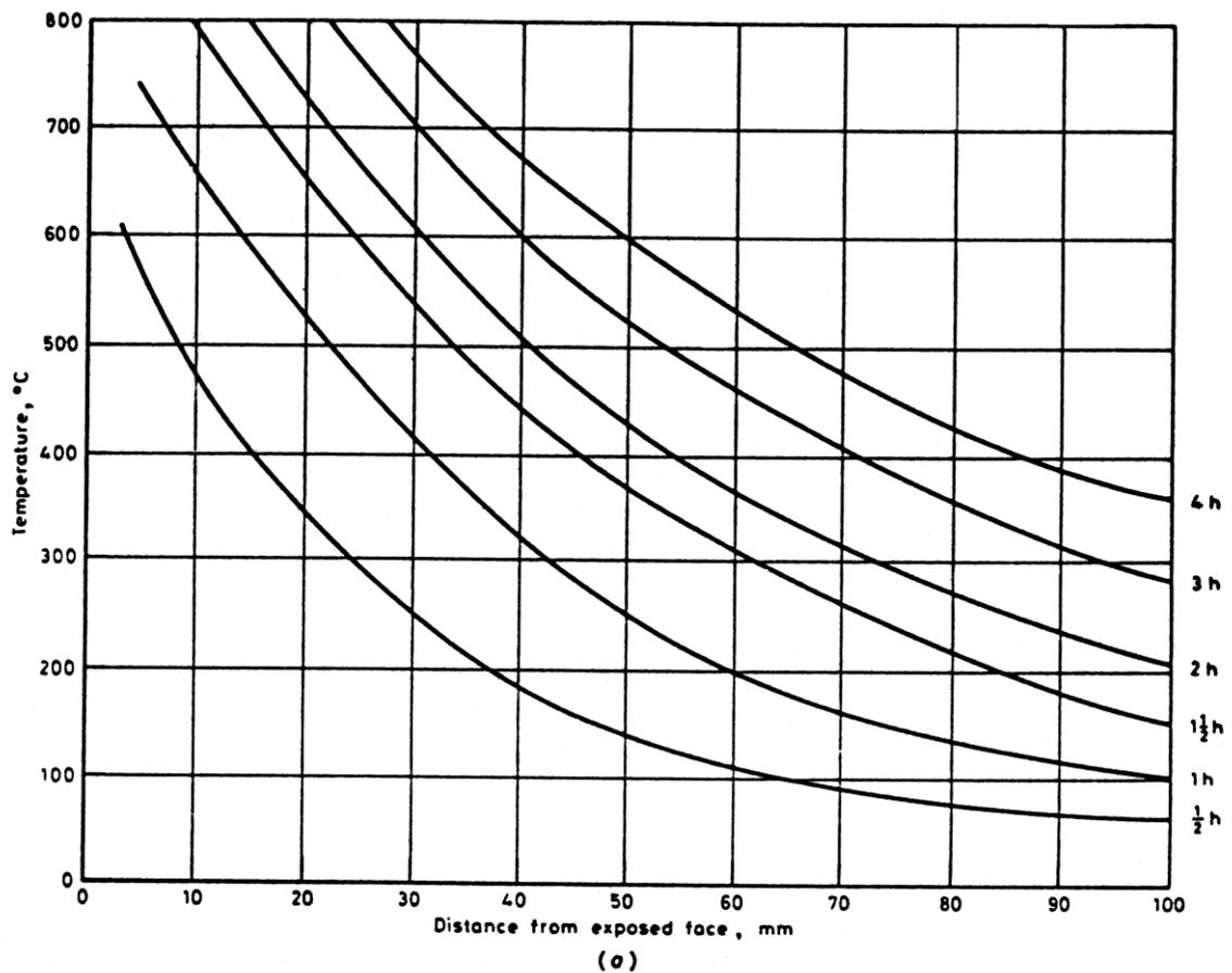
**Figure 2.11** Temperature distribution in a concrete slab for dense concrete [ISE(1978)]
