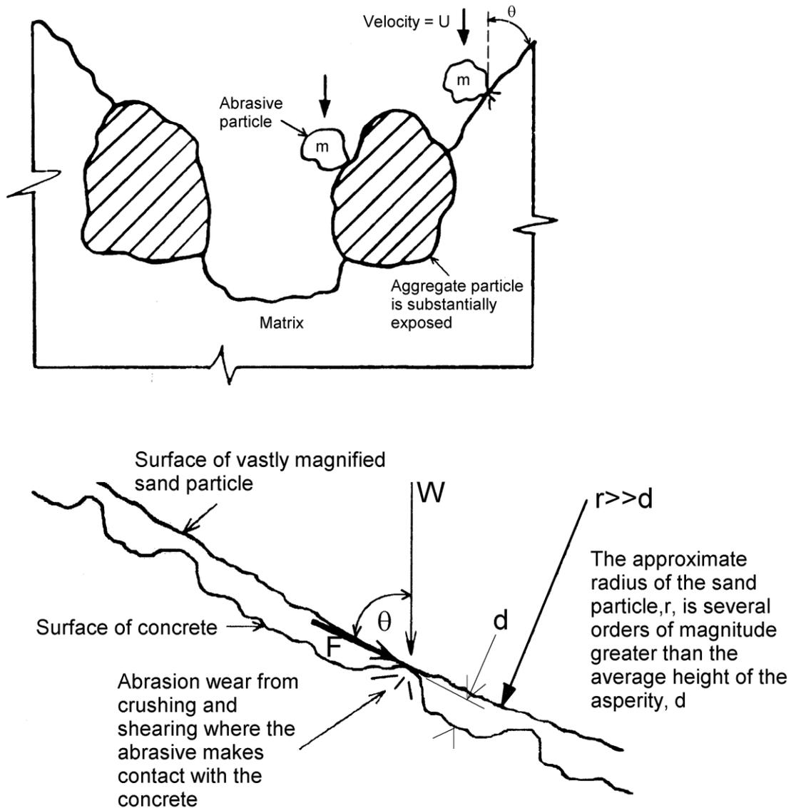
**Figure 4.4** (a) The abrasive sand is seen to impact against the surface at an angle  $\theta$ , causing microscopic crushing and shearing effects of the surface asperities, as seen in (b).
