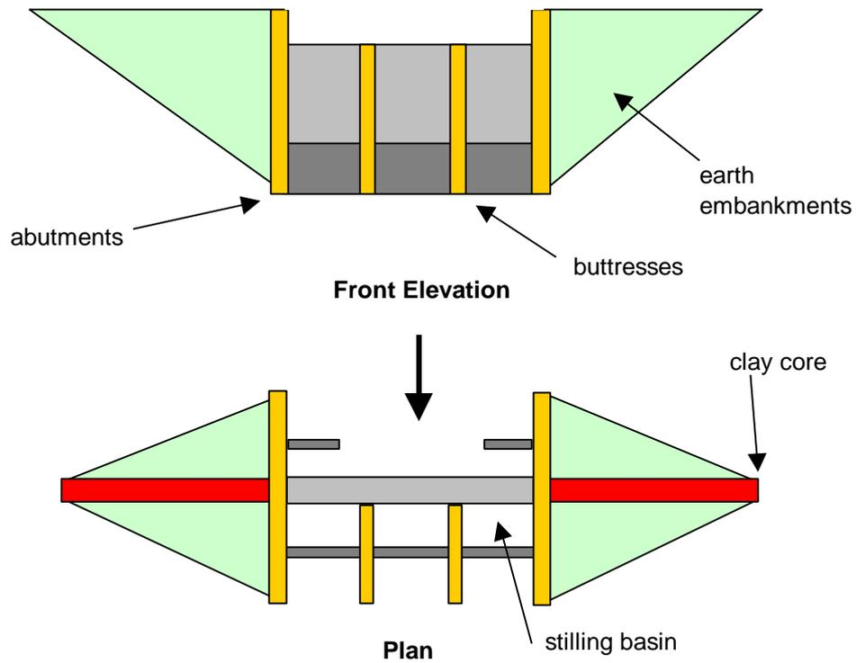
**Figure 6** – Plan and Front Elevation of proposed design
