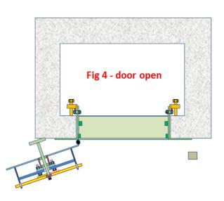
The retro-door is suitable for retro-fitting concrete vaults/bunkers where existing doors have been vandalised or stolen. See <a href="https://www.damsforafrica.com">www.damsforafrica.com</a> for other products in our range, which are variously suitable for securing pump-houses, sub-stations, valve-chambers, control panels, boreholes, etc.
