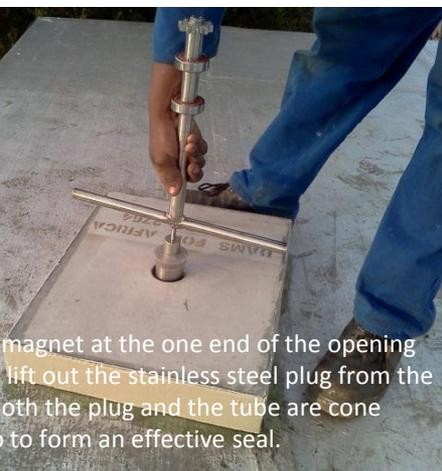
Figure 3 : With the plug removed the opening tool is inserted into the access tube – first the pinion, followed by the bearings to centralise the pinion.
