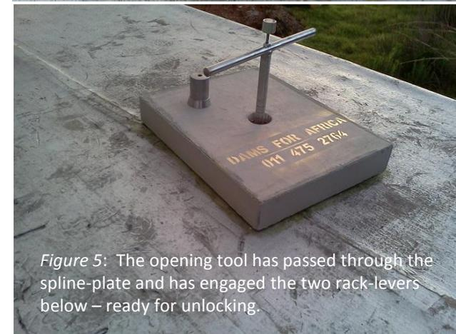
Figure 5: The opening tool has passed through the spline-plate and has engaged the two rack-levers below – ready for unlocking.
