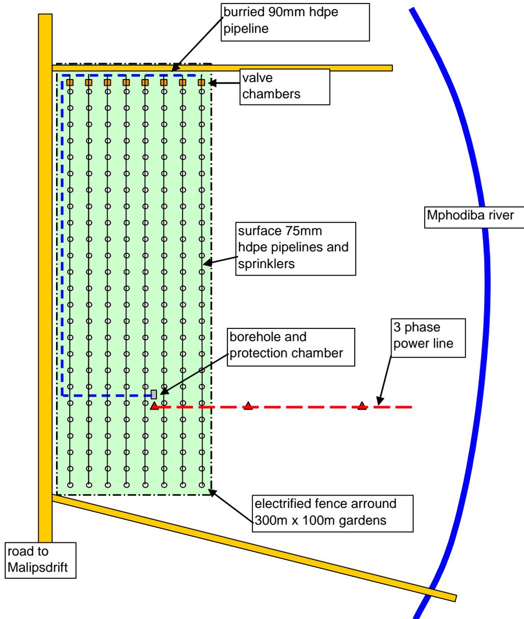
**Figure 3** – Plan of Irrigation system, power supply, and fencing, assuming 3 hectare option
