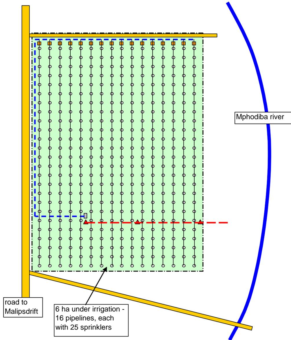
**Figure 5** – Plan of Irrigation system, power supply, fencing assuming 6 hectare option
