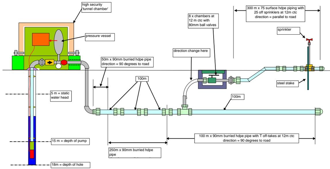
**Figure 4** – Typical section of irrigation system
